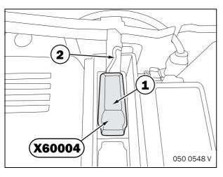
Fit connector housing (1) in position.
