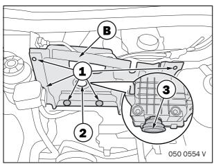
Secure partition  ${\bf B}$  using the screws (1) from the standard partition.
