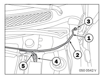
Pass black wire (1) from partition wiring harness **B** with cable lug through grommet (2) and connect at ground pin (3). Route cable (4) to recess (5).
