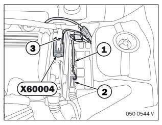
Route red wire (1) to fuse box and connect at PIN 8 of 12-pin connector (2). Fit cover to fuse box.
