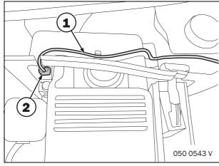
Route black wire (1) with 2-pin plug to the air cleaner and connect plug (2) to air cleaner.
