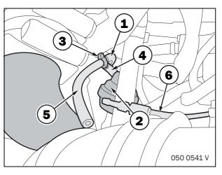
Detach hose from vacuum unit (2) on the compressor and connect to T-piece (3). Connect hose (4) to vacuum unit (2).
