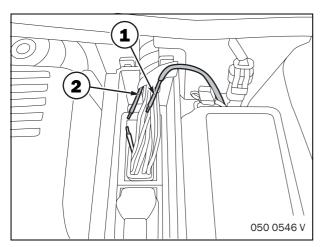
Connect (by twisting) yellow wire (1) to the one end (2) of the white/red wire.
