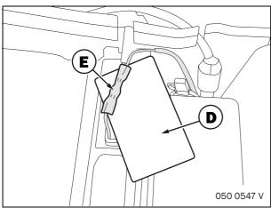
Connect white/red wire from connector and twisted wire with crimping pliers and crimp connector **E**. Make sure that the wires are connected correctly. Reconnect if necessary.
